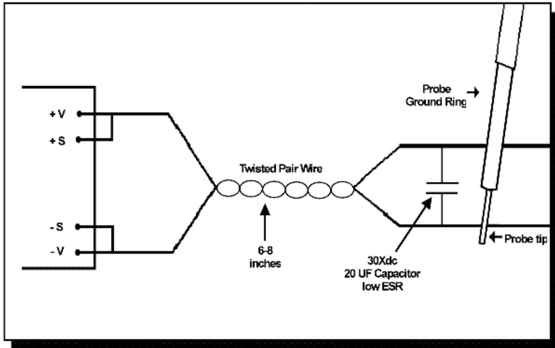
This test method will enable a remote measurement and eliminate any noise that may couple on to the extended leads coming off the converter.
