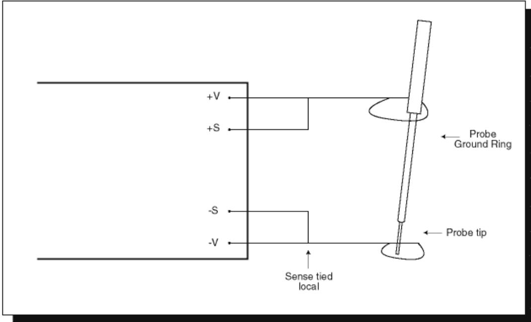
Utilizing the probe ground ring (as opposed to a ground wire) will minimize the chance of noise coupling from sources other than the power supply. If this is not practical or possible then attach a 6 to 8 inch twisted pair wire to the outputs of the power supply and place a 10-20 uF tantalum capacitor (low ESR type, with an appropriate voltage rating) across the load. This test method is shown on figure 1c.
